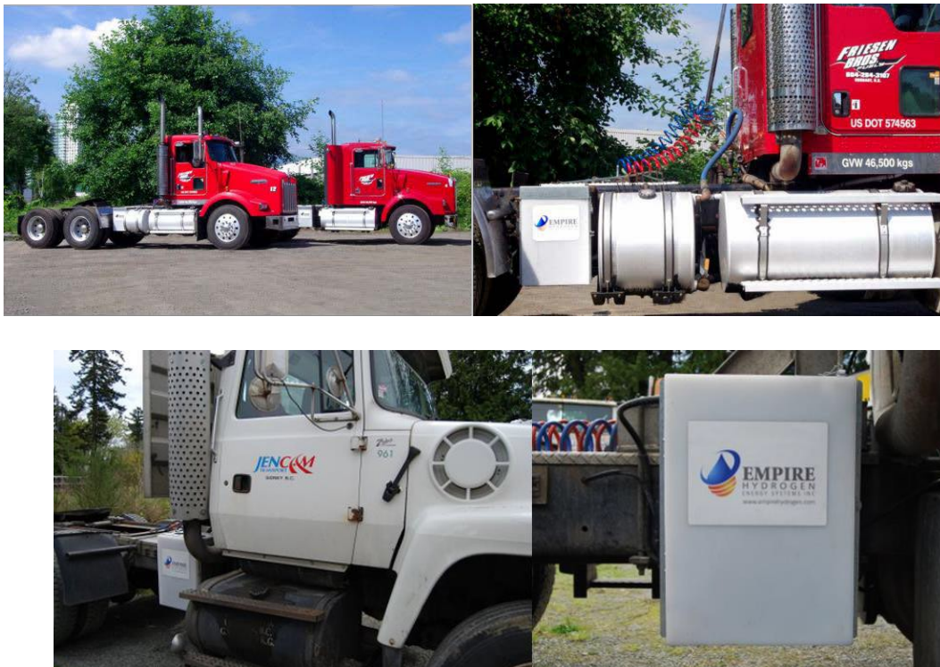
Jencam and Freisen Bros. Trucks used in APTDP – Displaying Mounted A/Gs
